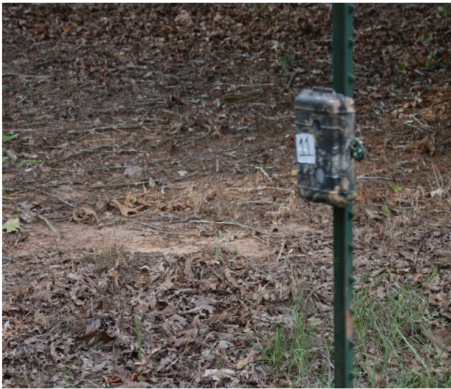
Figure 8. If necessary, use a t-post to correctly position cameras.
